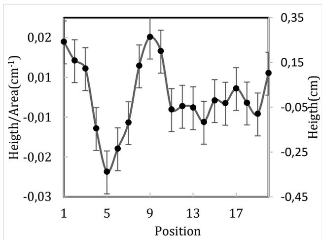
Fig. 3. Distance from the TA to the best fit plane vs point number (see point number in Fig. 2 c)). Values are expressed as Mean  $\pm$  Standard Error.
